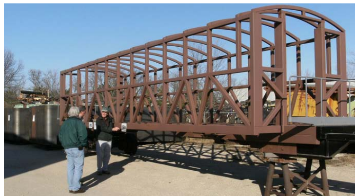
Here's the metal frame of the 'Officer's car' that will accompany the Lincoln Funeral car on tour in 2015. This car is patterned after the car pulled by the C&NW's first steam loco, the Pioneer, at the 1948 Chicago Railroad Fair.
