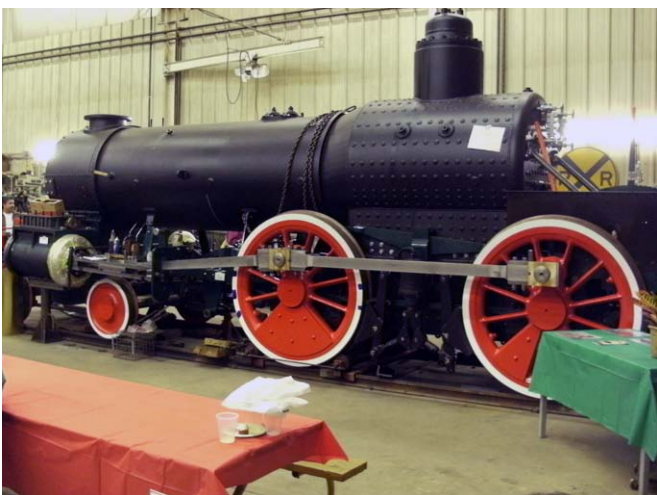
The 4-4-0 'York' will be completed in March. Then it heads east to a museum in York, Pennsylvania. The loco is sitting on small 40 lb. rail.
