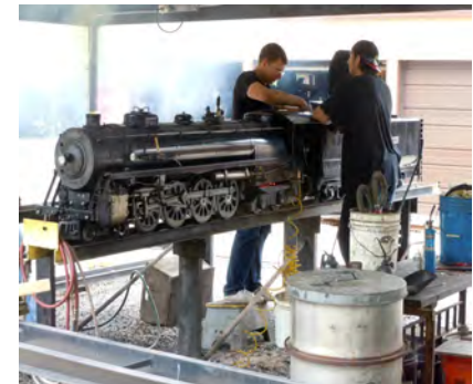
ILS crew members prep a big 4-8-4 steam engine for running. It took a good hour to fire this locomotive! Jim Osborn photo.
