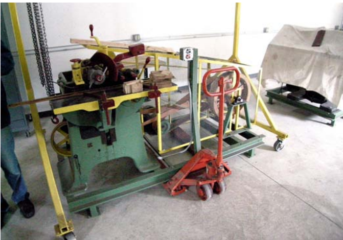
An older overhead belt driven shaper converted to electric drive and mounted on a portable platform.
