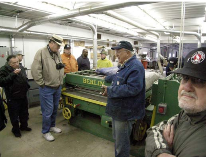
A three drum panel sander designed to finish sand doors and windows in one pass.
