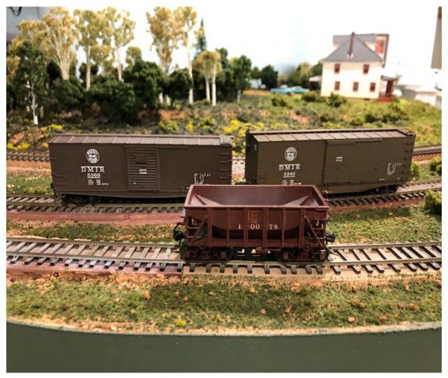
"I kit-bashed two "new" 36 foot DM&IR boxcars, both built pre-1910, that saw service into the 1960's. The steel car, 5366, received new steel doors on an MDC body, and the wood car, number 5240, is an Accurail kit that received new exterior fishbelly girders to match the prototype. The ore car is a 50 ton ore car which is smaller than all the 70 ton ore cars on my railroad. It started as a 3D printed body on an MDC ore car under frame with many added details." Bob Hanmer
