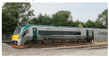
multiple unit diesel-electric sets where only the end units are powered. End units also have a control cab so the train does not need to be turned at terminals. They are geared for 100 mph and have been in use since 2008.
